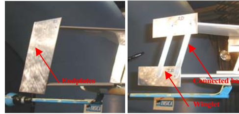
Figure 5.11: Endplate fixed and winglet+bar fixed
