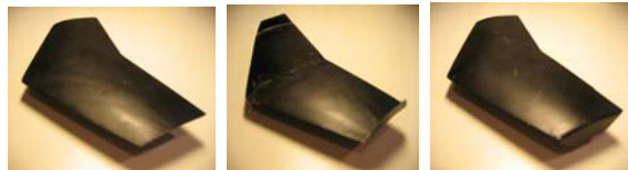
Figure 3.5: Curve plate wing model (A2.5S25.T0.6T0) Left: No winglet, Middle: Upper winglet, Right: Lower winglet
