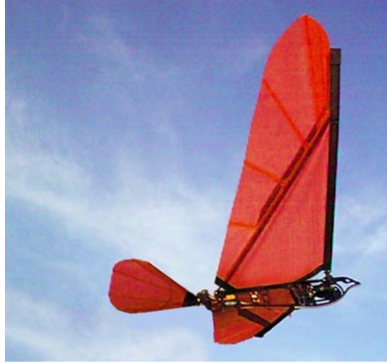
Figure 6: The Slow Hawk is a remote controlled aircraft available off-the-shelf ( http://www.ornithopter.org ). It has a wingspan of 150cm. It is 75cm long and weighs 510g. It can produce 4 wing beats per second and its maximum autonomy amounts to 12 minutes. To control this platform, three different channels are available: two concern the tail - they are used to keep the pitch and the roll - and one concerns the wing beat frequency. Only the dihedral is controlled. The sweep is constant and the twist is passively controlled by the tissue of the wings. This implementation simplifies wing structure but reduces the robot's maneuverability.
