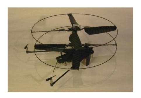
Coaxial rotor helicopter with 4 ch. radio control and a camera system. The yaw is gyro stabilized while the helicopter is utilizing a passively stable rotor system. The helicopter is operated by a remote pilot using feedback from the camera to help with the navigation when the helicopter is out of sight.
